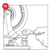
Tighten the adjustable stop bolts on the face and side arms down until they make contact with the guide base.
