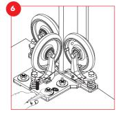
Securely tighten the mounting bolts and/or nuts (not included).
