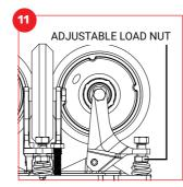
Loosen adjustable load nut on the face and side arms until the spring is no longer under compression.
