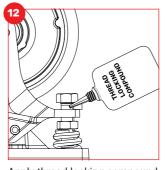
Apply thread locking compound to the adjustable stop bolt thread above the face and side arms, following manufacturer's instructions.
