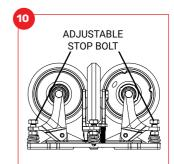
**Note:** This product has (3) adjustable stop bolts that are pre-set to provide the optimal float of 3 mm in post-to-post and back-to-front directions.
