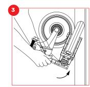
Hold the roller guide at an angle, positioning the face roller wheel onto the rail.
