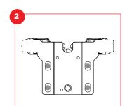
Verify the location of the mounting holes (refer to mounting template).
