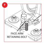
Remove the face arm retaining bolt so the face roller wheel preload is applied to the rail.
