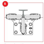
Ensure the guides are aligned correctly (as shown) before making any further adjustments.
