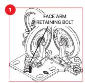
The Calibre C-150 roller guide comes completely assembled with the preload set on each wheel
