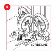
Roll guide down until positioned over the mounting holes or studs.
