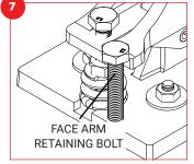
Remove the face arm retaining bolt Securely tighten the mounting bolts and/or nuts. Mounting hardware is to attain the factory set pre-load on the face arm roller wheel.
