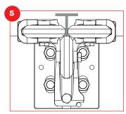
Be sure that guides are aligned properly (as shown) with the face and side roller wheels touching the rail, before making any further adjustments.
