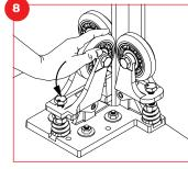
At this point, there will be 11 - 23 kg (25 - 50 lbs) of pressure on each side roller wheel and the face roller wheel, and it will be possible to skid the roller wheels by hand with moderate effort.
