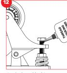
Loosen adjustable load nut on the face and side arms until the spring is no longer under compression.
