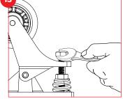
Tighten the adjustable stop bolts on the face and side arms down until they make contact with the quide base.
