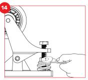
Tighten the adjustable load nuts on the face and side arms down until they make contact with the side or face arm springs and prevent them from rattling, but do not compress them
