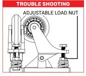
If fine tuning of the roller wheel pressure is required, proceed with the step below.
