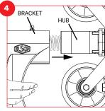
Place bracket onto the hub of wheel cluster assembly.
