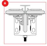
Be sure guides are aligned properly (as shown) before making any further adjustments.
