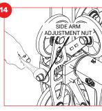
Adjust side arm roller wheel pressure. Turn side arm adjustment nuts until side roller wheels are compressed 1/32" - 1/16" (1-2 mm), and face wheels are tracking in the center of the rail.
