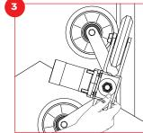
Position the uppermost roller wheels of wheel cluster assembly onto the rail, and while maintaining pressure against the rail, roll entire assembly upward until face roller wheels are firmly seated on the rail.
