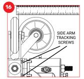
Each pair of side arm roller wheels should track parallel to the face of the rail. The distance from the edge of each roller wheel to the face edge of the rail should be the same at both the top and bottom wheels of each pair.
