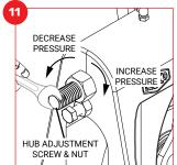
To adjust the wheel pressure on the rail, back the hub adjustment nut off about half way down the hub adjustment screw. Turn the hub adjusting screw in 4 turns. This represents approximately 50 lbs (25 kg) of wheel pressure
