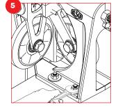
Position bracket over mounting holes or studs. Align the front face of the rail with the scribe line. Install mounting hardware (not included with guide) as required. Tighten lightly to hold bracket in place prior to final adjustment.
