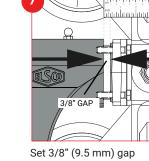
between wheel cluster assembly and bracket following the markings on the hub.
