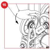
At this point, there will be 25 - 50 lbs (12 - 25 kg) of pressure on each side roller wheel and the wheels can be skidded by hand on the rail with moderate effort.
