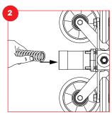
After verifying the proper location of the mounting holes (refer to mounting template), insert the spring into the hub.
