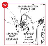
If fine tuning for float adjustment is required, turn the adjustable stop screw clockwise to decrease float or, turn adjustable stop screw counterclockwise to increase float.
