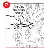
If it is necessary to adjust the side arm tracking, turn the side arm tracking screws until top and bottom roller wheels are parallel to the face rail
