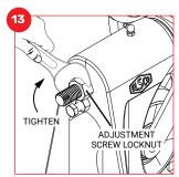
When properly adjusted, it will be possible to skid the face roller wheel by hand with moderate effort.
