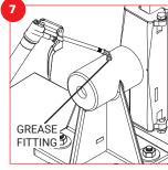
At this point, install the remaining guides on top of and/or beneath the elevator. Lubricate the fitting on each guide with general purpose grease until a small amount appears between the hub and bracket.
