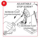
To limit postwise float, turn adjustable stop screw clockwise until it makes contact with solid stop washer (installed in step 2).
