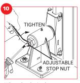
When the desired amount of postwise float is set, tighten the adjustable stop locknut securely while holding adjustable stop screw in place.
