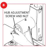
Insert adjustable stop kit and and nut into bracket. The hub adjustment screw regulates the pressure of the gib against the face of the rail. The stop adjustment screw regulates the postwise float of the car.
