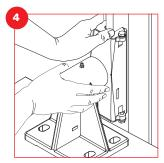
Position swivel sliding guide shoe onto the rail while lowering mounting bracket over the mounting holes or studs. Install mounting hardware (not included).
