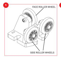
The Model E Guide comes completely assembled.
