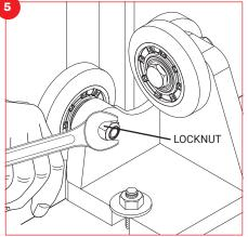
Adjust side roller wheel pressures in the same manner as step 4, while keeping the face roller wheel tracking in the center of the rail. When the side roller wheels are properly positioned, tighten locknuts.
