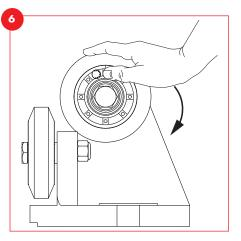
When properly adjusted, all roller wheels should be compressed 1/32" - 1/16" (1 - 2 mm), which represents approximately 25 - 50 lbs (12 - 25 kg) of wheel pressure. At this pressure, it will be possible to skid the roller wheels by hand with moderate effort.
