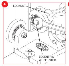
To adjust face roller wheel, loosen locknut and turn the eccentric wheel stud to increase or decrease wheel pressure against the rail. When the face roller wheel is properly positioned, tighten locknut.
