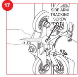
If it is necessary to adjust side arm tracking, loosen and turn side arm tracking screws until top and bottom roller wheels are parallel to the face of the rail.
