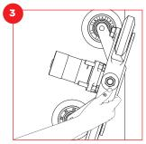
Position uppermost roller wheels of wheel cluster assembly onto the rail, and while maintaining pressure against the rail, roll entire assembly upward until face roller wheels are firmly seated on the rail.
