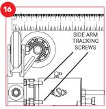
Each pair of side arm roller wheels should track parallel to the face of the rail. The distance from the edge of each roller wheel to the face edge of the rail should be the same at both the top and bottom roller wheels of each pair.
