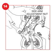
Adjust side arm roller pressure. Turn side arm adjustment nuts until side wheels are compressed 1/32" - 1/16" (1-2 mm) and the face wheels are tracking in the center of the rail.
