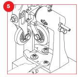
Position bracket over mounting holes or studs. Install mounting hardware (not included with guide) as required. Tighten lightly to hold bracket in place prior to final adjustment.
