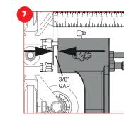
Set 3/8" (9.5 mm) gap between wheel cluster assembly and bracket following the markings on the hub.
