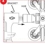
If you separated the wheel cluster assembly to install first, next you will place the bracket onto the hub of wheel cluster assembly.
