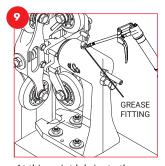
At this point lubricate the fitting on each guide with general purpose grease until a small amount appears between the hub and the bracket.
