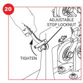
When the desired amount of postwise float is set, tighten the adjustable stop locknut securely while holding adjustable stop screw in place.
