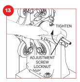
Be certain that both the face wheel pressure and the recommended gap measurement (refer to step 7) are equal for each guide. Now tighten the hub adjustment screw locknut.
