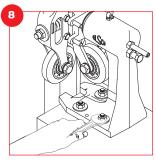
Securely tighten mounting bolts. Repeat steps 7 and 8 on remaining guides before proceeding. This helps assure that the elevator car will be properly centered between the rails.
