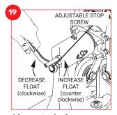
If fine tuning for float adjustment is required, turn the adjustable stop screw clockwise to decrease float or, turn adjustable stop screw counterclockwise to increase float.
