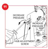
Turn the hub adjustment screw in 3.5 turns. This represents approximately 50 lbs (25 kg) of wheel pressure.
