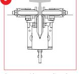
Be sure guides are aligned properly (as shown) before making any further adjustments.
