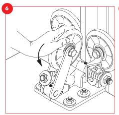
When properly adjusted, it will be possible to skid the face roller wheel by hand with moderate effort. Be certain that the face roller wheel pressures are equal for each guide.
