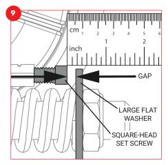
To adjust float, turn the square-head set screw to increase or decrease the gap between the large flat washer and the head of the squarehead set screw.
