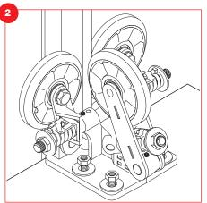
Position guide base over mounting holes or studs. Install mounting hardware (not included). Make certain that the centers of the front mounting slots are located two inches (51mm) back from the face of the rail (refer to mounting specifications).
