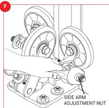
Adjust side roller wheel pressure. Turn the side arm adjustment nuts until side arm wheels are compressed 1/32" - 1/16" (1-2 mm), and the face arm wheels are tracking in the center of rail. This represents approximately 25-50 lbs (12-25 kg) of roller wheel pressure on each side arm wheel.
