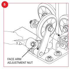
To adjust face roller wheel pressure, tighten face arm adjustment nut until the wheel is compressed 1/32" - 1/16" (1-2 mm). This represents 25-50 lbs (12-25 kg) of roller wheel pressure.
