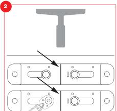
Place ASME-compliant mounting hardware (customer supplied) through slots and mounting surface. Align notches on brackets with center of face rail. Use torque wrench to tighten bolts to 160 ft-lbs to prevent slippage and hardware damage.
