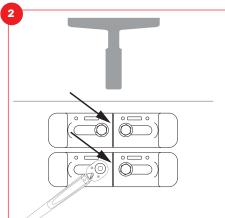
Place ASME-compliant mounting hardware (customer supplied) through slots and mounting surface. Align notches on brackets with center of face rail. Use torque wrench to tighten bolts to 80 ft-lbs to prevent slippage and hardware damage.
