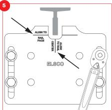
Position plate onto brackets and align notches on plate throat to rail. Use torque wrench to tighten provided bolts to 160 ft-lbs.
