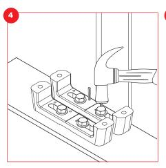
Using hammer, install narrow end of 1-1/4" tapered pins in newly-drilled holes (outer or inner holes only).
