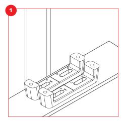
Clean mounting surface to remove any grease, debris, etc. Center elevator car. Position brackets onto mounting surface to confirm slots and mounting holes match.
