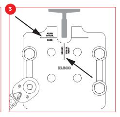
Position plate onto brackets and align notches on plate throat to rail. Use torque wrench to tighten provided bolts to 80 ft-lbs.
