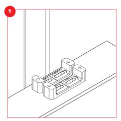
Clean mounting surface to remove any grease, debris, etc. Position brackets onto mounting surface to confirm slots and mounting holes match.
