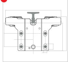
Verify the proper location of the mounting holes (refer to mounting template).
