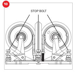
**Note:** This product has (3) stop bolts that are pre-set at the factory for optimized float of 3 mm (1/8") in post-to-post and back-to-front directions.
