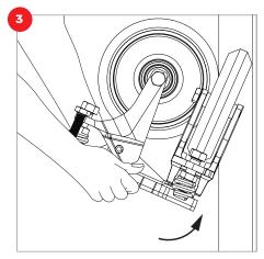
Hold the roller guide at an angle, positioning the face roller wheel onto the rail, and while maintaining pressure against the rail, roll the entire assembly upward until the side arm roller wheels engage with the rail.
