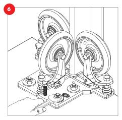
Securely tighten the mounting bolts and/or nuts. Mounting hardware is not included.
