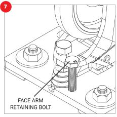
Remove the face arm retaining bolt to attain the factory set pre-load on the face arm roller wheel.
