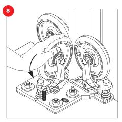
At this point, there will be 9-27 kg (20-60 lbs) of pressure on each side roller wheel and the face roller wheel.
