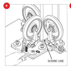
Roll guide down until positioned over the mounting holes or studs. Ensure that the front face of the rail is aligned with the scribe line.
